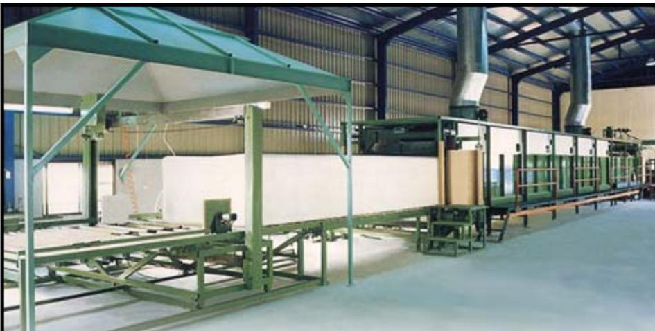
A foam slabstock machine. Source: [www.foam-cutting-machinery.com](http://www.foam-cutting-machinery.com)
